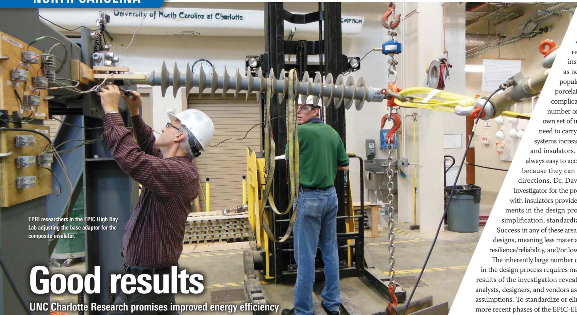
EPRI researchers in the EPIC High Bay Lab adjusting the base adaptor for the composite insulator.
