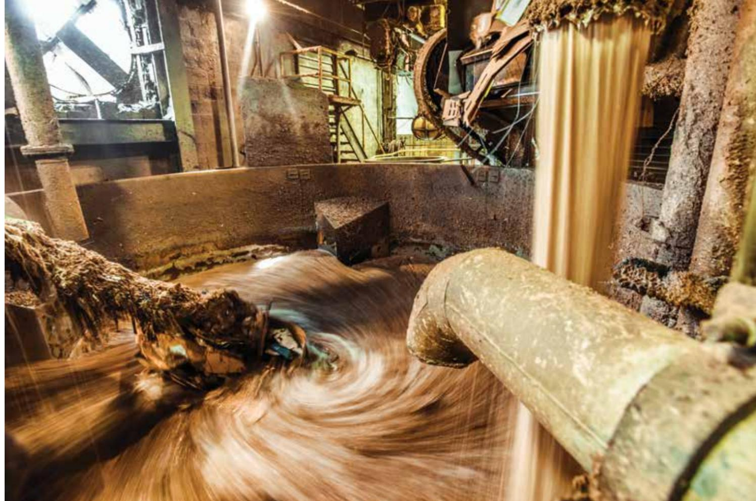
A machine resembling an enormous blender churns used boxes into pulp, with the help of about 900,000 gallons of recycled water.
