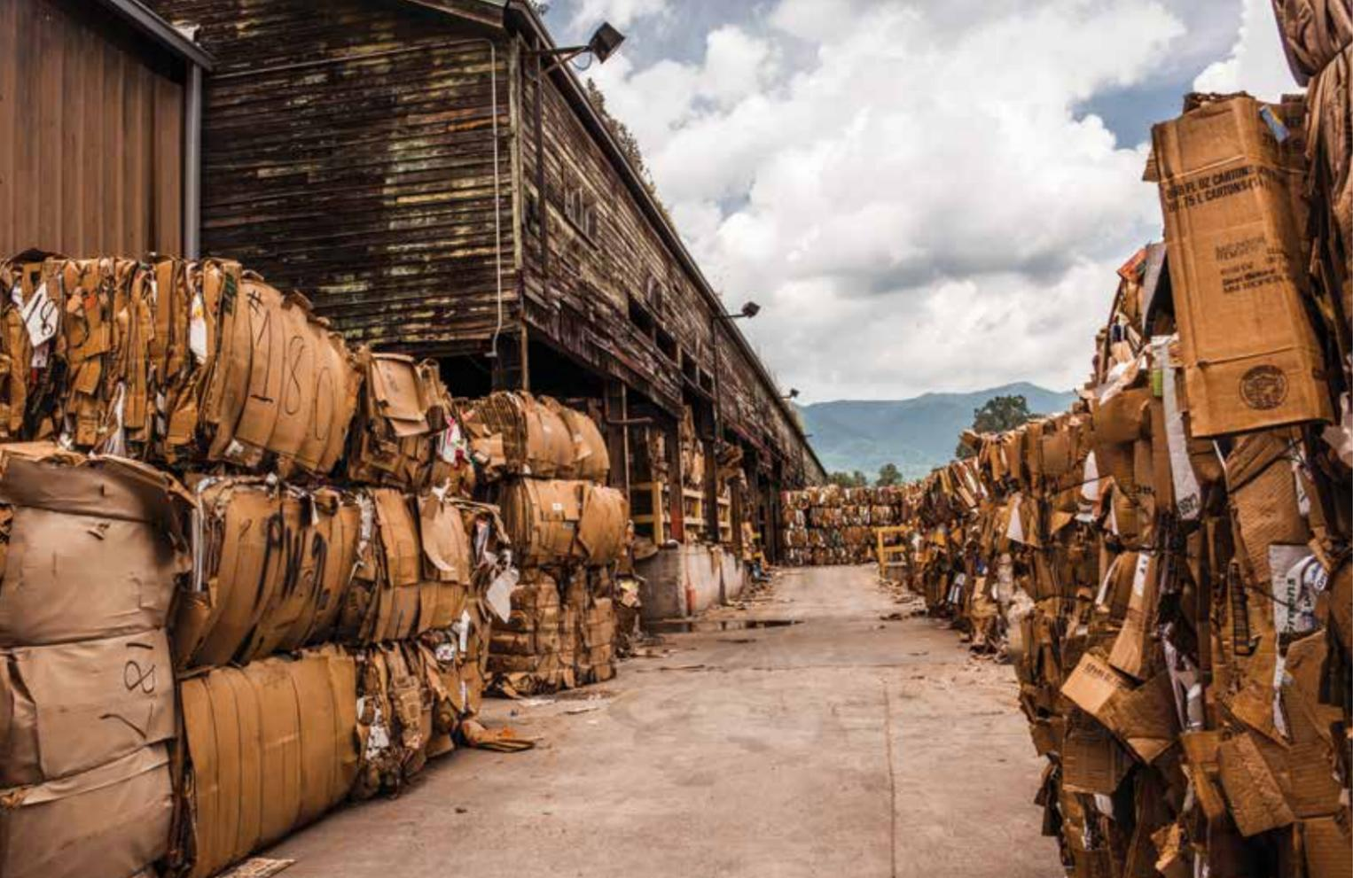
More than 100,000 tons of recycled corrugated containers are trucked in, cleaned and cooked into new sheets of paper every year at Jackson Paper in Sylva.
