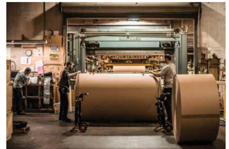
Rolls are cut to the customer's desired width, about 20 to 110 inches.
